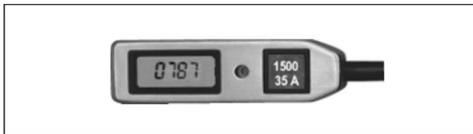
Figure 3-16. Example of Military CYPRES Control Unit Setting
